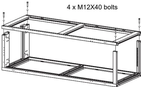
If during assembly of the side upright the holes are not aligned or if there is a space of 4mm between the uprights, it is required to loosen the bolts and reassemble.
