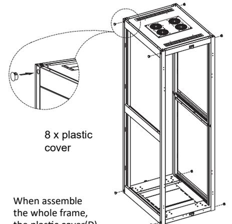
When assemble the whole frame, the plastic cover(D) should be removed.
