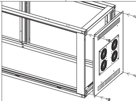
For the cabinet over 800 depth, the fans should be assembled closed to the rear door.
