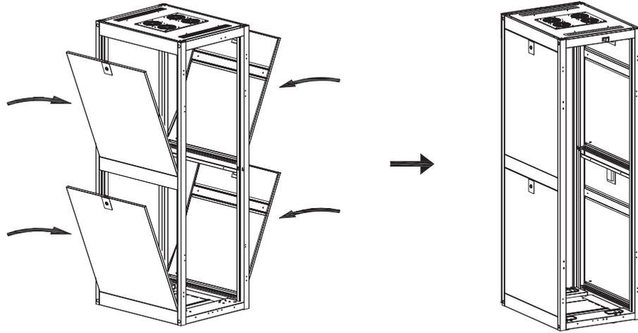
Single or double doors can be fitted front and rear - (Normally single door at the Front and double doors at the rear).
