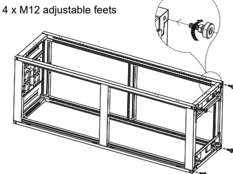
After assembling, the M12 feet should be under (shorter than) the castors in case of breaking when set up the cabinet!
