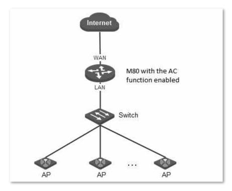
The AC management function of M80 allows you to configure wireless settings, advanced settings, manage APs and view user status.
