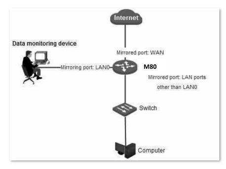
The mirroring port of M80 is fixed to LAN0 and cannot be changed.
