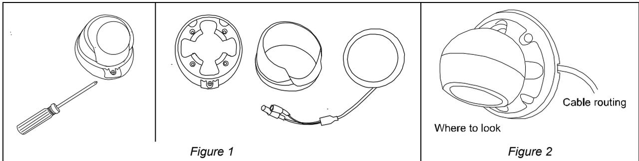
Step3: Drill 4 holes and screw the base to the wall (or ceiling).
