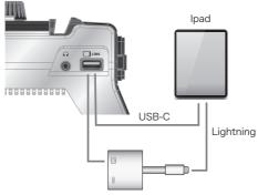
\*Note: For iPad with USB-C connector, simply connect the USB-A to USB-C cable to the UC9020. Or use the USB-A to USB-A cable along with an Apple Lightning USB 3 Adapter (not included, may need additional purchase) to iPad with the lightning connector.
