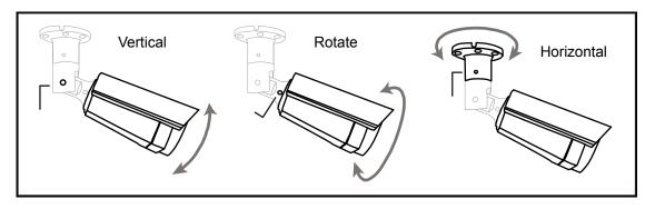
Step 3: Power on the camera and fine-tune the viewing angle.
