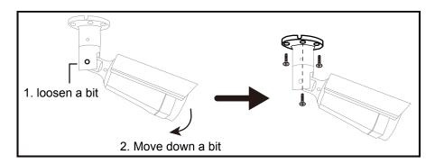
Step 2: Adjust the viewing angle of the camera as indicated below.
