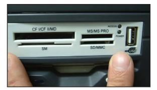
4. Secure the Multi-Card Reader/Writer in place on both sides using the enclosed mounting screws.
