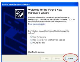
Insert the included driver CD in your CD-ROM drive and make your connection to a USB port. When the Welcome to the Found New Hardware Wizard screen displays (above), click "Cancel" to continue with the installation.
