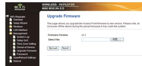
After a firmware upgrade file is selected, click '**Upload**' button, and the router will start firmware upgrade procedure automatically. The procedure may take several minutes, please be patient.
