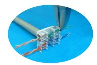
Follow the cap color code to place the wires into the cap slot. Keep the pairs twisted as possible as you can and cut off the surplus wires.
